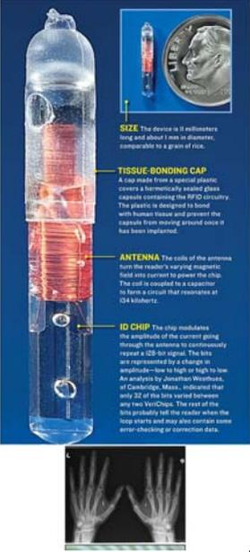
**SIZE** The device is 2 millimeters long and about 1 mm in diameter, comparable to a grain of rice.
